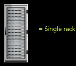
16 Nodes 200TB/node @ 85% compression Single rack / data center floor tile
